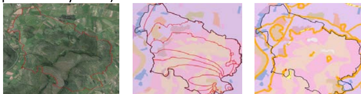
Fig. 4. The orange and red bands indicate the buffer zones for the application of the fuel load reduction. The coloured lines (red, violet, green, cyan) indicate the fire propagation for each simulation, the time step is 30'.
